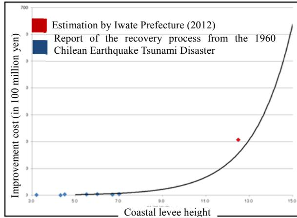
**Figure 5 Coastal levee improvement cost**
